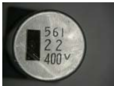
Marking code is different than spec and should be 250V – counterfeit
